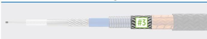
A braid's function is usually to provide extra tensile strength and RF shielding to the cable. However, in this instance the main function is slightly different, in aiding the positioning of the spring layer. For the spring to maintain its position along the cable – to not expand nor rotate when torsion is applied and to exert resistance to any crush forces – it must be prevented from bunching and shifting along the cable. The braid serves as a reinforcement mechanism to prevent such movement.
