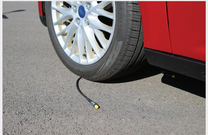
*In the charts that follow, the blue trace is the initial state and the red trace shows the performance of the cable after being run over by the car 10 times.*
