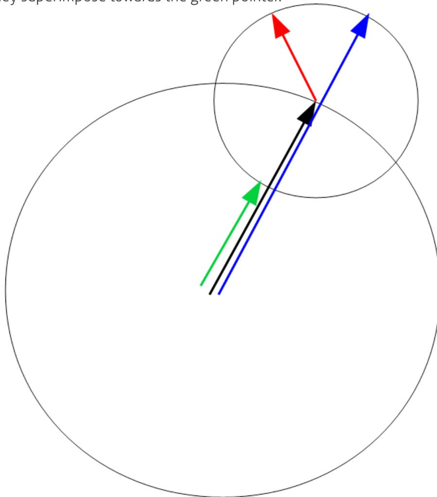
*Fig. 1: Superposition of signals with different phase (and different voltage)*
