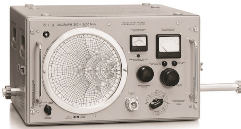
Fig. 5: Zg-Diagraph manufactured by Rohde und Schwarz
